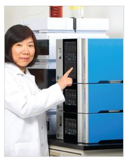
Wyatt Technology, a specialist in dynamic light-scattering instrumentation, has demonstrated that a combination of sizeexclusion chromatography, a multiangle light-scattering platform, and ultraviolet and differential refractive index detectors can be used to assess the quality of adenoassociated virus gene therapy vectors.
