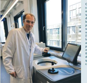
Coriolis Pharma, a contract research organization that specializes in formulation development of biopharmaceuticals, performs sedimentation velocity ultracentrifugation (SV-AUC) experiments to assess the quality of adeno-associated virus preparations. Pertinent measurements include the relative amounts of differently sedimenting species (filled and empty capsids).
