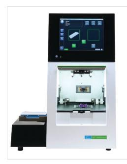
The PerkinElmer LabChip GXII Touch, an instrument for performing protein and nucleic acid analysis, can distinguish differences of protein molecular weight as low as 1 kDa. By reproducibly and accurately measuring capsid composition, the instrument can facilitate the characterization of recombinant viral particles, a crucial step in gene therapy applications.
